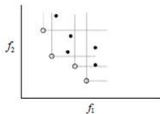
Figure 3.3: The Pareto Optimal frontier is the set of hollow points. Operational decisions must be restricted along this set if operational efficiency is to be maintained
