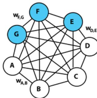
Figure 3.7: Graphical representation for a Boltzmann machine with a few labelled weights
