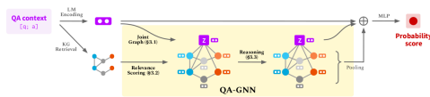
Figure 8: QAGNN architecture: Retrieved KG is connected to the QA context and relevance of KG nodes is computed conditioned on the QA context. Post per-node relevance scoring, reasoning is done over the entire graph. (Yasunaga et al., 2021)
