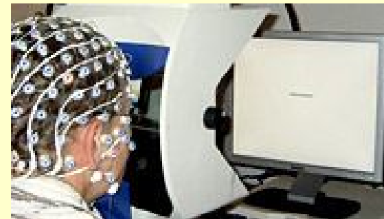
A bit more complicated way to measure gaze using electric potential around the eye.
