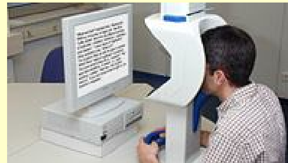
The ergonomic chin rest eye tracking device for high speed and accurate measurements with a large visual field.
